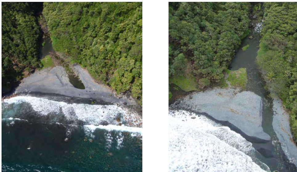
Figure 5. Two photographs of the mouth of Kopili'ula Stream, Maui. The image on the left shows a closed stream mouth berm and the image on the right show the berm open. Notice the lower stream discharge on the left (i.e., more exposed rocks in stream and no white water in the upper riffle) as compared to the higher discharge on the right.
